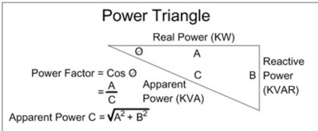
This simple illustration shows that in an inductive environment, capacitors provide capacitive reactance, which can eliminate the need for reactive power supplied from the source. As a result, one of the byproducts of a capacitive reactance is a reduction in Total Apparent Power. Another way to demonstrate this is that capacitors are used for phase correction; reducing  $\theta$  which in turn increases power factor and reduces Total Apparent Power.
