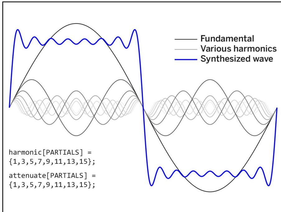
Total harmonic distortion (THD) is a common measurement of the level of harmonic distortion present in a power system. THD is defined as the ratio of total harmonics to the value of the fundamental frequency and is calculated as:
